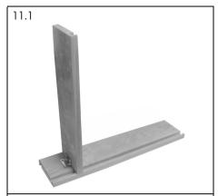
Fit the rear of the drawer (J) to one of the drawer sides (H) and fix into position using the long screws (R) provided.
