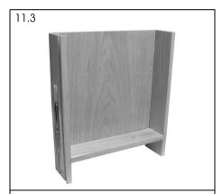
Rotate the drawer and slide the drawer base (I) into position.
