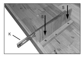
7. Fit the legs into position and secure the assembly using long machine screws (S).
